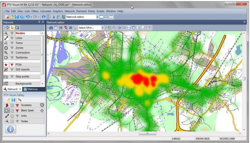
PTV Visum Safety generates a heat map based on user accident data to focus road safety action programs on the significant areas e.g. cyclists.
