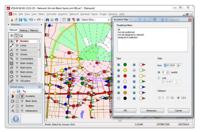
The accident data can be filtered depending on the accident main attributes. Easy filtering of accidents with cyclists.
