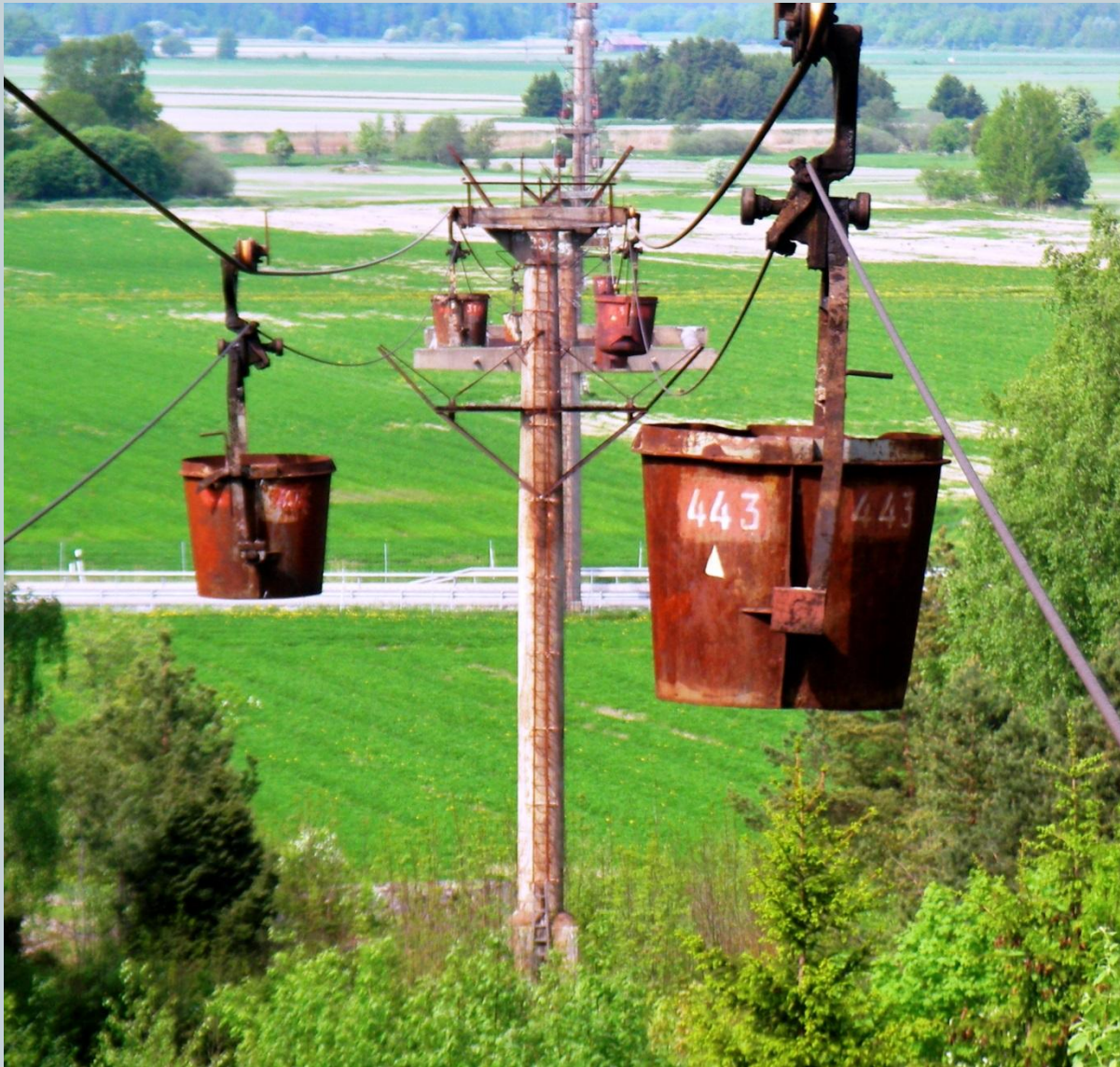
Ropeway conveyor for Limestone transportation in Sweden
