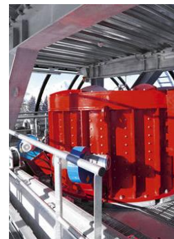
GEARLESS DRIVE SYSTEM DIRECTDRIVE
