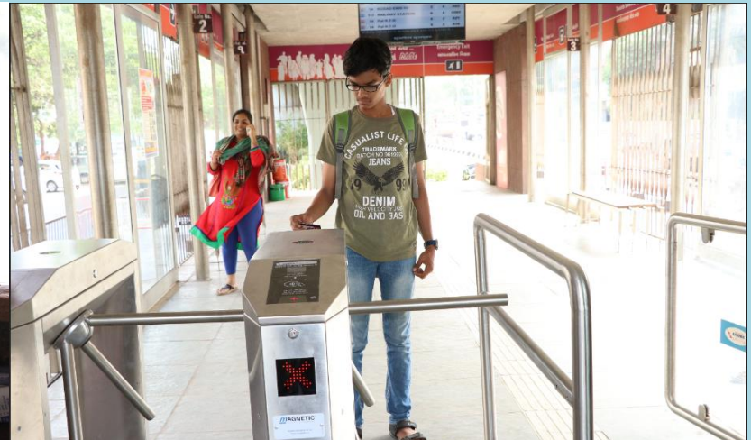
Turnstile with Fare gate Validator
