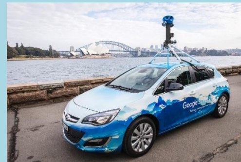
GOOGLE STREET VIEW CAR WITH MOUNTED CAMERAS
