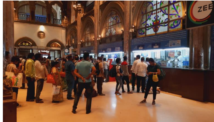
No accessible (low height) counter provision; lacking tactile guidance provisions
